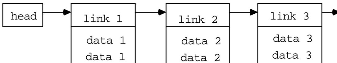
information in addition to the link. A list of them might be drawn like this: The 'head' is a pointer to the first element. This could be stored in a memory location, or in a register in the ARM. The first field in each element is the link pointer, and this is followed by two data words. The pointer for the third element does not point anywhere; it marks the end of the list.
