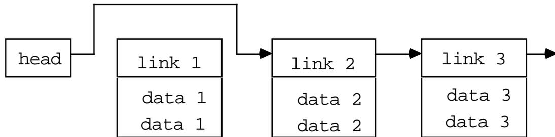
Notice that item number one is now inaccessible through the list, so in order to use it, a pointer to it must be 'remembered' somewhere. Notice also that if the item removed was the last one, the head pointer would be given the end of list value, and would not point at anything. This is known as an empty list.
